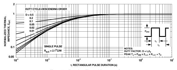
Figure 13. Transient Thermal Response Curve
