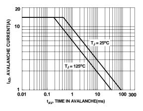
Figure 9. Unclamped Inductive Switching Capability
