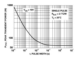
Figure 12. Single Pulse Maximum Power Dissipation
