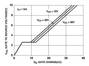
Figure 7. Gate Charge Characteristics
