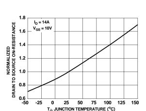
Figure 3. Normalized On-Resistance vs Junction Temperature
